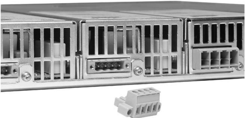
Figure 5. Quick disconnects for power and sense leads
